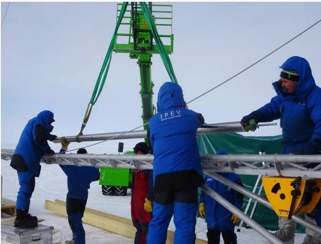
Fig. 5 The SUBGLACIOR probe being positioned in its berth before deployment in the test borehole at Concordia station.
